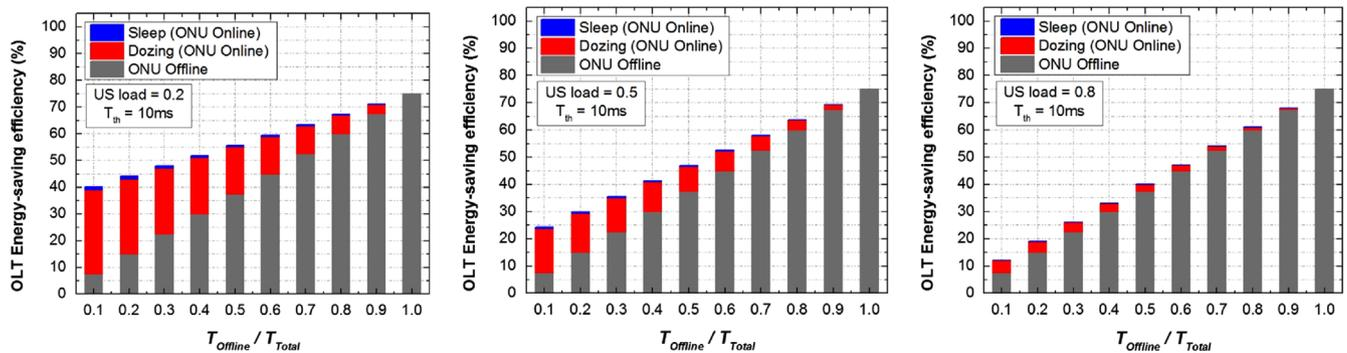
Fig. 10. OLT energy-saving efficiency versus  $T_{Offline}/T_{Total}$ .
