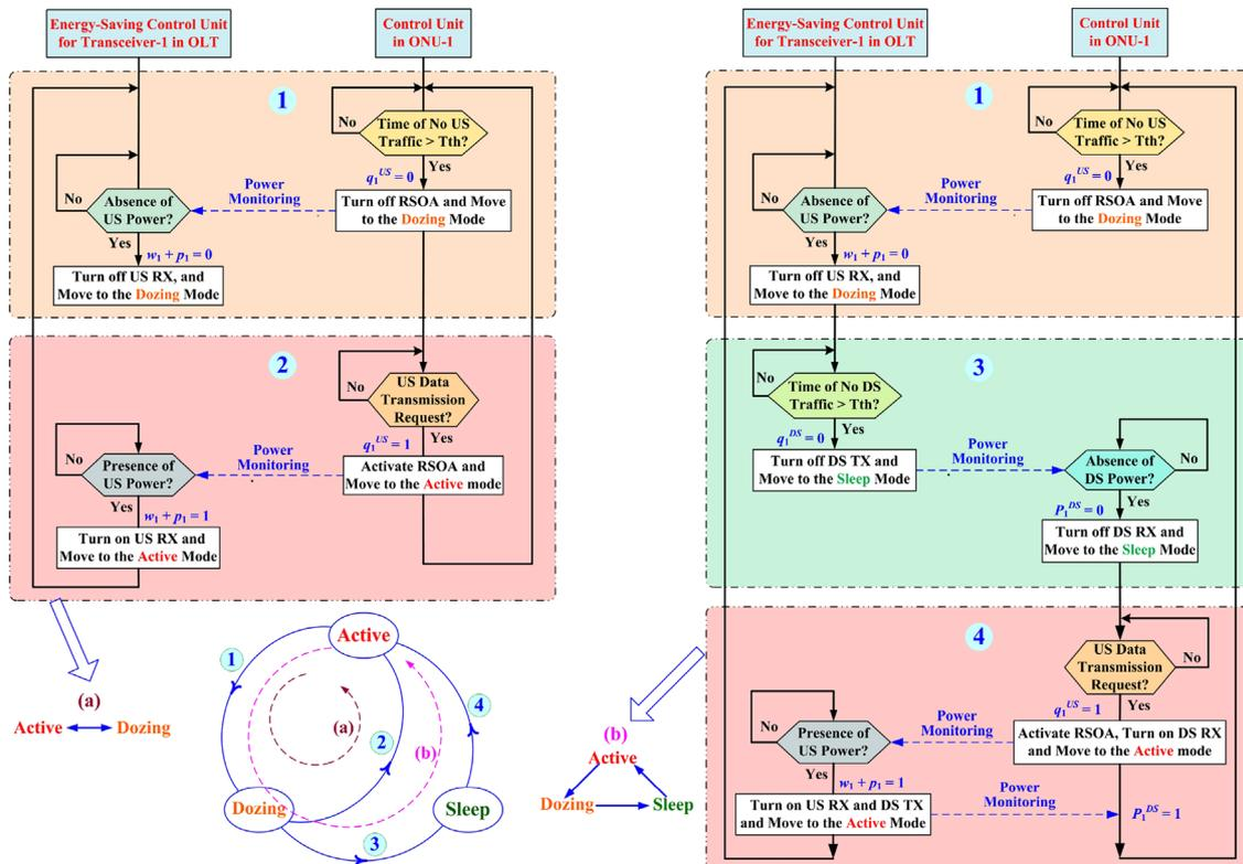
Fig. 2. The two possible sequences (a) and (b) of state transitions for ONU-1 and Transceiver-1 in the OLT in our proposed energy-saving scheme.
