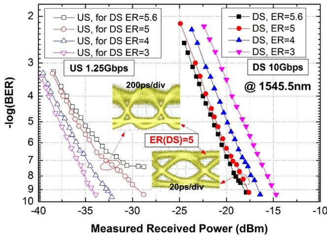
Fig. 4. Measured BER of the DS and US signals at 1545.5 nm for different DS ERs. Insets show the optical eye patterns when the DS ER is 5 dB.
