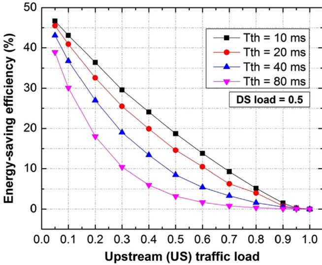
Fig. 6. Energy-saving efficiency as a function of US traffic load for different time thresholds by using our proposed energy-saving scheme.
