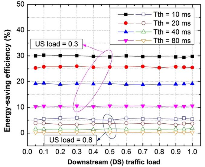
Fig. 7. Energy-saving efficiency versus DS traffic load under different time thresholds and different US traffic loads.
