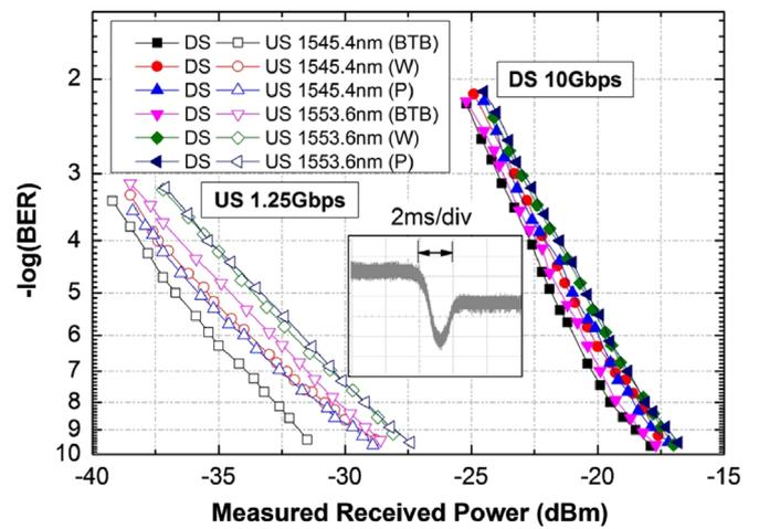
Fig. 5. Measured BER of the 10 Gbit/s DS and 1.25 Gbit/s US signals both in the working and protection modes at 1545.5 nm and 1553.6 nm. Inset shows the switching time during traffic restoration.
