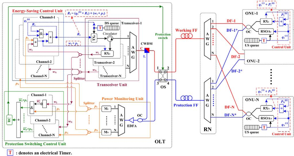
Fig. 1. Schematic diagram of the CLS-based WDM-PON architecture with the proposed energy-saving and centrally-controlled self-healing scheme.
