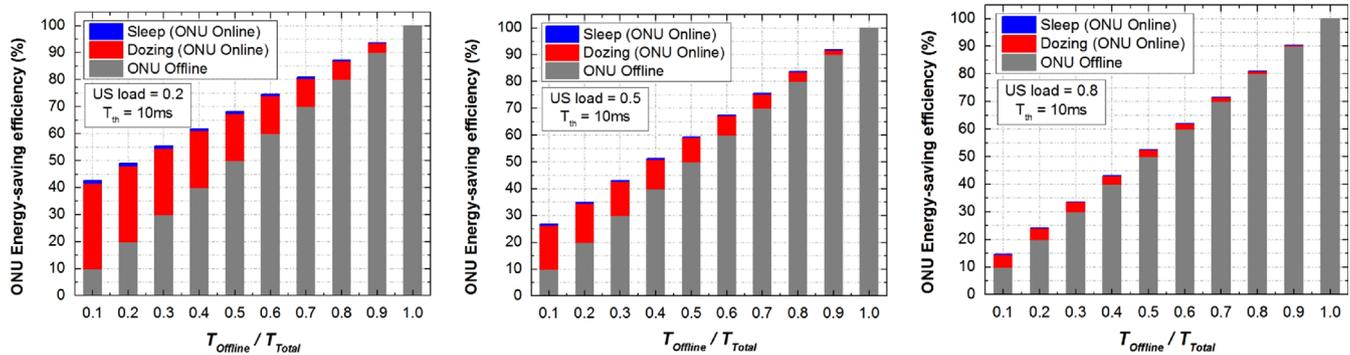
Fig. 9. ONU energy-saving efficiency versus  $T_{Offline}/T_{Total}$ .
