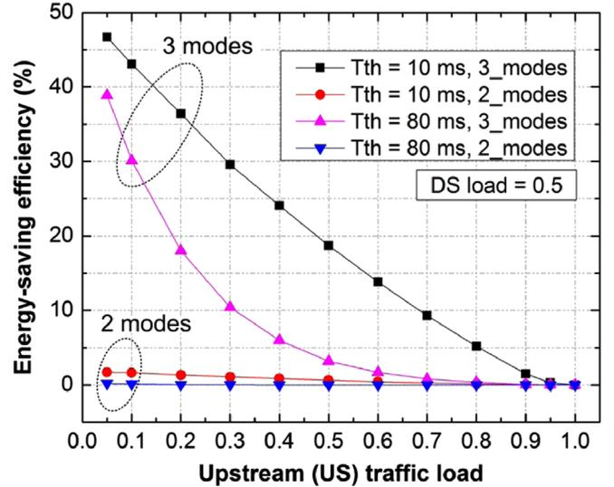
Fig. 8. Comparison of energy-saving efficiencies for our proposed 3-mode scheme and those 2-mode schemes in [11–13] under different time thresholds.
