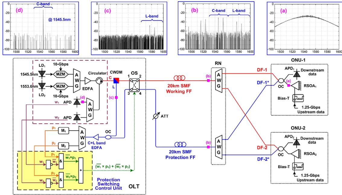
Fig. 3. Experimental setup for the centrally-controlled self-healing operation in the proposed WDM-PON architecture.
