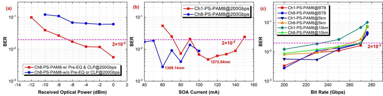
Fig. 3. (a) the BER versus ROP for BTB case w/o and w/ Pre-EQ or clipping process in the channel 8; (b) the measured BER versus SOA current in the channel 1 and 8; (c) the BER versus different bit rates with different cases in the channel 1 and 8.
