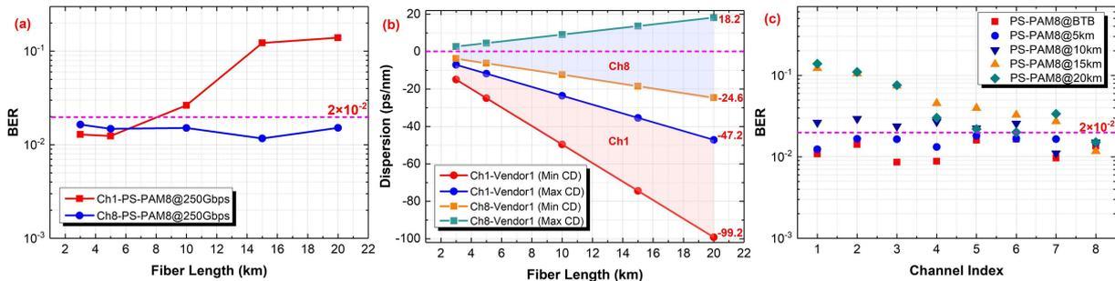
Fig. 4. (a) the BER versus Fiber Length in the channel 1 and 8; (b) the maximum and minimum chromatic dispersion versus Fiber Length for the channel 1 and 8; (c) the BER versus different channels after different transmission cases.
