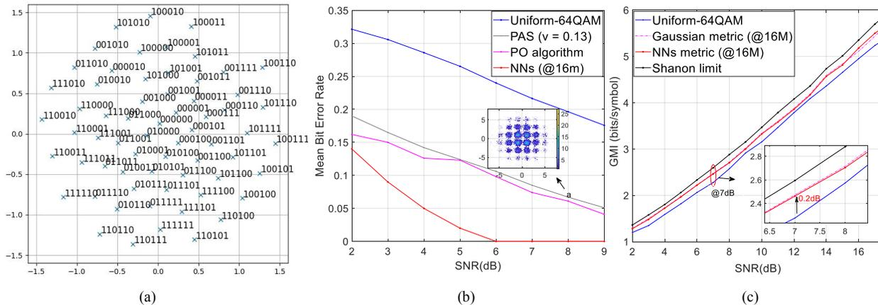
Fig. 3. (a) Geometric constellation optimization of 64QAM including Gray-like mapping; (b) Mean BER comparison against SNR; (c) GMI performance comparison against SNR.
