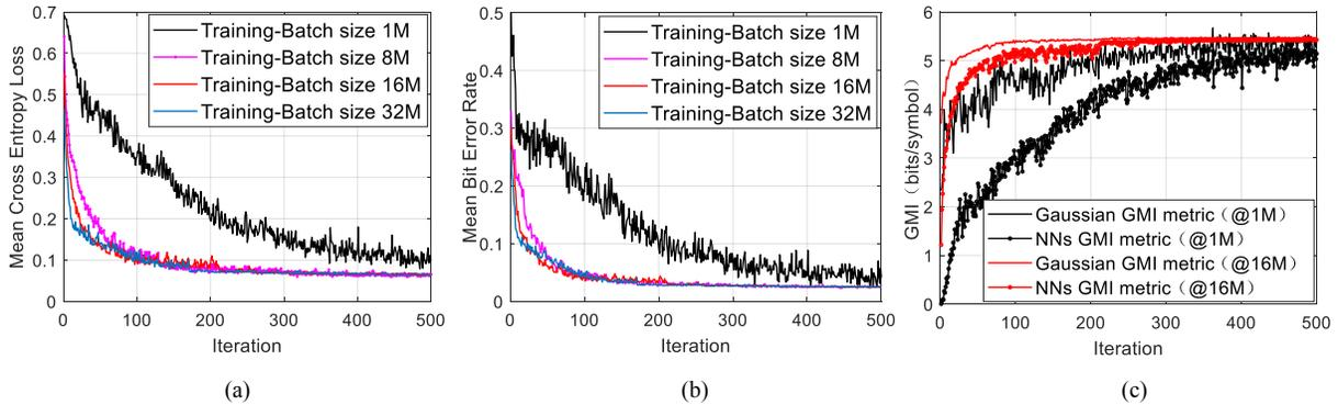
Fig. 2. (a) Convergence of mean cross entropy loss for different batch sizes; (b) Convergence of mean BER for different batch sizes; (c) GMI performance comparison for Gaussian metric and NNs metric.
