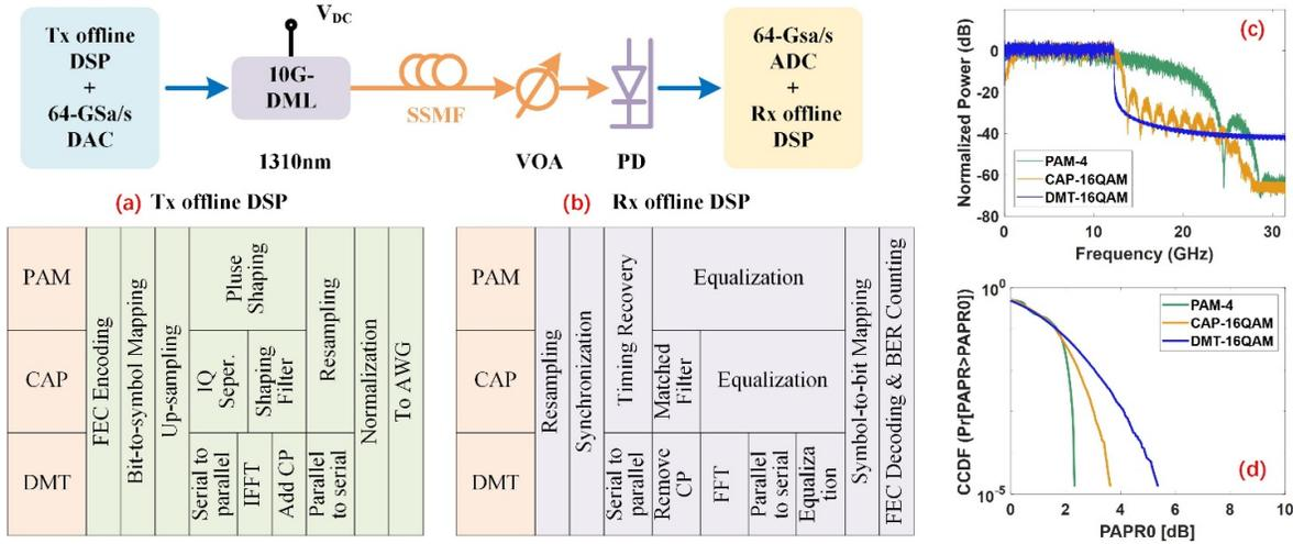
Fig. 1. Simulation setup for 50-Gb/s PON system based on bandwidth-limited optics at O-band: (a) and (b) Tx and Rx offline DSPs, (c) spectra and (d) PAPR for PAM-4, CAP-16QAM and DMT-16QAM signals, respectively.
