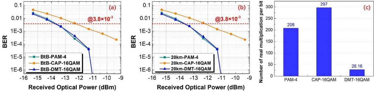
Fig. 3. BER versus ROP for 50-Gb/s/λ PON with different formats: (a) BtB; (b) 20 km; (c) Computational complexity of three modulation formats.
