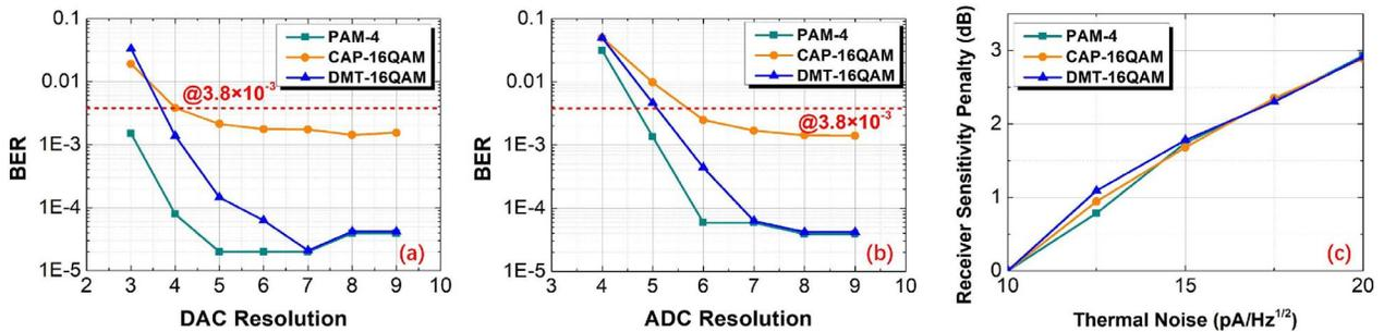
Fig. 2. (a) BER versus DAC resolution; (b) BER versus ADC resolution; (c) Receiver sensitivity penalty versus thermal noise.
